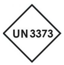
The UN mark must be of sufficient size that each side has a length of at least 50mm, the width of the line must be at least 2mm and the letters and numbers must be at least 6mm high.
